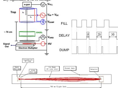
**Figure 1.** [not to scale] (Left) Schematic of experimental apparatus. (Right) A timing diagram for the data acquisition sequence that leads to time-resolved TOF spectra. (Bottom) For the data presented here the trap assembly was floated (~200V) above ground and an Einzel lens was installed about 15 cm above the electron multiplier assembly to improve the mass resolution and detection efficiency of the apparatus.
